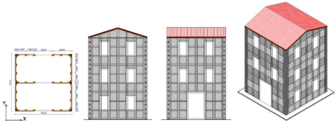
Fig. 11 Case study: modular wall panel arrangement
